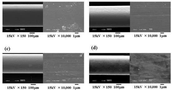
**Figure 7.** Scanning electron microscopy images of each wire before and after friction tests (**a**) surface of 19-25PEEK before friction test; (**b**) surface of 19-25PEEK after friction test; (**c**) surfaces of Ni-Ti before friction test; (**d**) surface of Ni-Ti after friction test.
