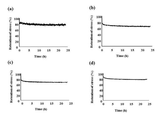
**Figure 5.** Rate of retention stress (**a**) rate of retention stress of 16 PEEK (Polyetheretherketone); (**b**) rate of retention stress of 16-22PEEK; (**c**) rate of retention stress of 19-25PEEK; (**d**) rate of retention stress of Ni-Ti.
