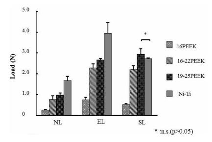
**Figure 2.** Load values of each wire at a maximum deflection of 2000  $\mu$ m for the respective ligation methods.
