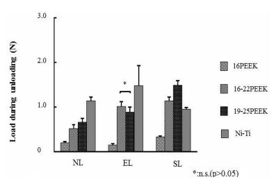
**Figure 3.** Load values of each wire at a deflection of 1500  $\mu$ m during unloading for the respective ligation methods.
