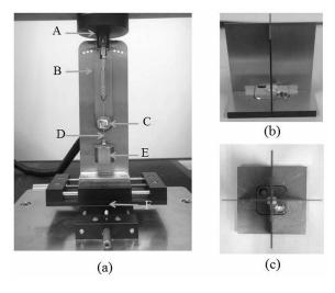
**Figure 12.** Friction testing systems (**a**) friction-testing device. A: load cell, B: base plate; C: bracket bonded stainless steel plate, D: wire, E: 150-g weight, and F: x-y table. (**b**,**c**) bracket-mounting device.
