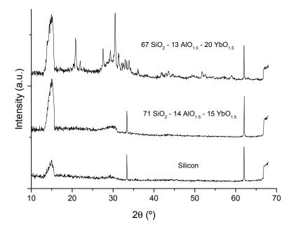
**Figure 2.** X-ray diffraction patterns of silicon and two aluminosilicate films with 15 and 20 mol%  $YbO_{1.5}$ , heat treated at 1100 °C.
