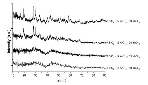
**Figure 1.** X-ray diffraction patterns of sol-gel derived Yb-doped aluminosilicate bulk samples, heat treated at 1050 °C.
