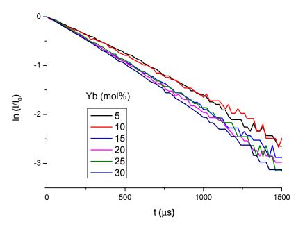
Figure 7. PL decay curves of aluminosilicate bulk glass samples doped with 5–30 mol% YbO<sub>1.5</sub>.
