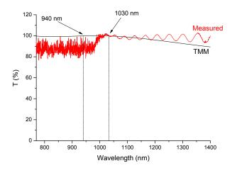
**Figure 9.** Transmission of an anti-reflective coating (ARC) with 3 layers deposited on 71 SiO<sub>2</sub>-14 AlO<sub>1.5</sub>-15 YbO<sub>1.5</sub> glass film deposited on silicon substrate, compared with TMM simulation.
