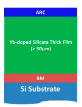
Figure 14. Schematic structure of the active disks prepared.
