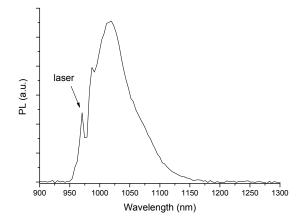
**Figure 13.** PL emission spectrum of an active disk (BM/71 SiO<sub>2</sub>-14 AlO<sub>1.5</sub>-15 YbO<sub>1.5</sub> film, 36.3  $\mu$ m thick/ARC), excited at 970 nm.
