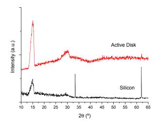
**Figure 11.** X-ray diffraction patterns of an active disk (BM/36.3  $\mu$ m thick 71 SiO<sub>2</sub>-14 AlO<sub>1.5</sub>-15 YbO<sub>1.5</sub> film/ARC) on a silicon substrate.
