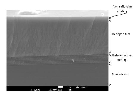
**Figure 10.** FEG-SEM cross section micrograph of a ~10  $\mu$ m thick active disk doped with 15 mol% YbO<sub>1.5</sub>, obtained in secondary electron mode. (Scale bar = 1  $\mu$ m).
