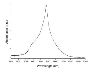
Figure 4. Near infrared absorption spectrum of 79 SiO<sub>2</sub>-16 AlO<sub>1.5</sub>-5 YbO<sub>1.5</sub> bulk gel.
