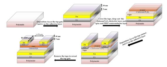
Figure 1. The fabrication process of the bottom-gate top-contact flexible organic thin-film transistor.
