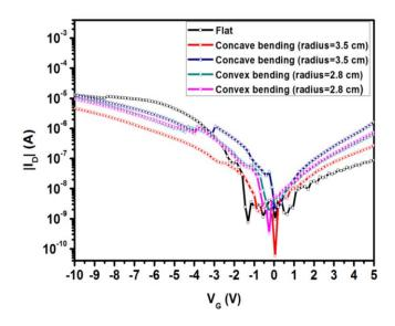
**Figure 8.** Comparison of the electrical characterization of the P3HT-based organic thin-film transistors (OTFTs) with a 0.023 wt % blended  $Y_2O_3$ /chitosan dielectric gate for bending tests at different bending radii and without bending.
