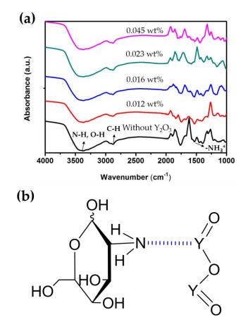
**Figure 7.** (a) FTIR spectra of the blended  $Y_2O_3$ /chitosan thin films; (b) Schematic diagram of hydrogen bonding between the  $Y_2O_3$  nanoparticles and the amine group of chitosan.
