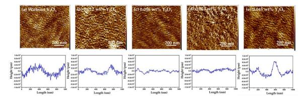
**Figure 4.** AFM morphology and profile depth of the pinholes in the surface of the  $Y_2O_3$ /chitosan thin film with various  $Y_2O_3$  concentrations: (**a**) Without  $Y_2O_3$ ; (**b**) 0.012 wt %; (**c**) 0.016 wt %; (**d**) 0.023 wt %; and (**e**) 0.045 wt %.
