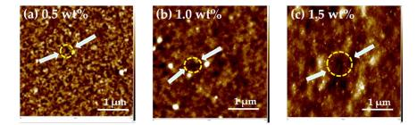
**Figure 2.** (**a**) 0.5 wt % chitosan shows many small holes (**b**) 1.0 wt % chitosan shows a few middle-sized holes and (**c**) 1.5 wt % chitosan shows many large holes.
