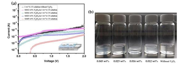
**Figure 3.** (a) Leakage current of the thin films measured with various concentrations of  $Y_2O_3$  solutions (without  $Y_2O_3$ , 0.012 wt %, 0.016 wt %, 0.023 wt %, 0.045 wt %) in 1 wt % chitosan solution (b) Pictures showing the various weight percentages of  $Y_2O_3$  in the mixed solution.
