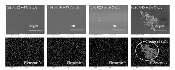
**Figure 6.** EDX images showing the distribution of yttrium: (**a**) 0.012 wt %; (**b**) 0.016 wt %; (**c**) 0.023 wt %; and (**d**) 0.045 wt %.
