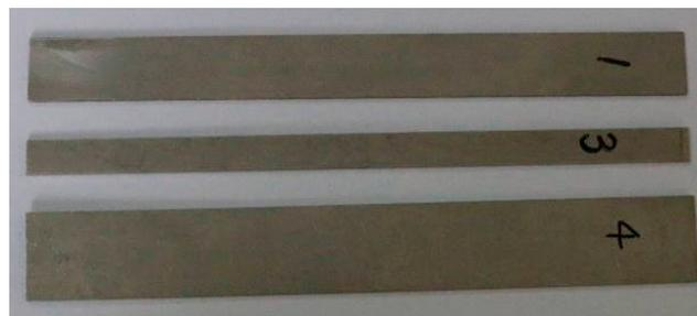
**Figure 11.** Waveguide bars named by No. 1, No. 3 and No. 4 (the width of No. 1 is 15 mm, No. 3 is 7 mm, and No. 4 is 20 mm).
