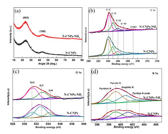
**Figure 2.** (a) XRD patterns of the N-CNPs and N-CNPs-NH<sub>3</sub> samples. High-resolution XPS spectra. (b) C 1s; (c) O 1s; and (d) N 1s bands of N-CNPs and N-CNPs-NH<sub>3</sub>.
