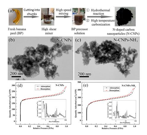
**Figure 1.** (a) Description of process from fresh banana peels to porous carbon. TEM images of (b) N-CNPs and (c) N-CNPs-NH<sub>3</sub>. Nitrogen sorption isotherms and the corresponding pore size distributions of (d) N-CNPs and (e) N-CNPs-NH<sub>3</sub>.
