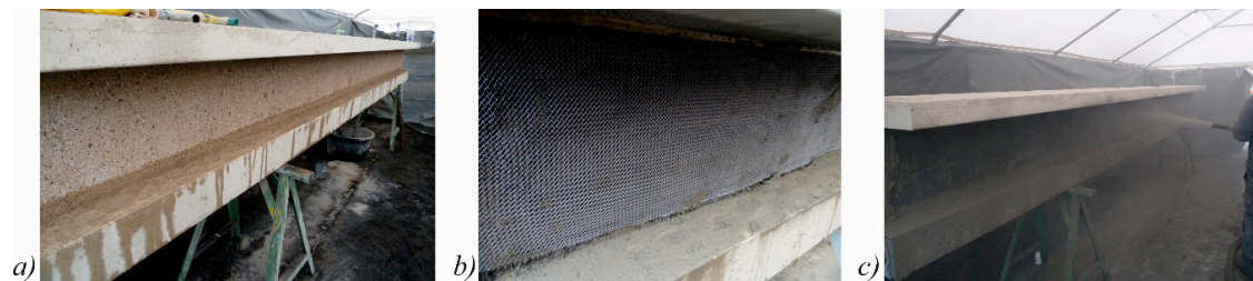
Figure 10. (a) Test specimen after shot blasting; (b) the application of the textile reinforcement; and (c) the application of shotcrete layers.
