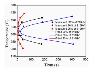
**Figure 11.** The time-temperature-property (TTP) curves of the studied alloy subjected to have been solid solution treated at 470 °C for 1 h, isothermal heat treatment for various durations, and then aged at 120 °C for 24 h.
