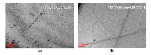
**Figure 8.** BF images of the studied alloy having been isothermal heat treated at 445 °C for different durations (5 s and 30 min), and then aged at 120 °C for 24 h. The isothermal heat treatment durations are: (**a**) 5 s; (**b**) 30 min.
