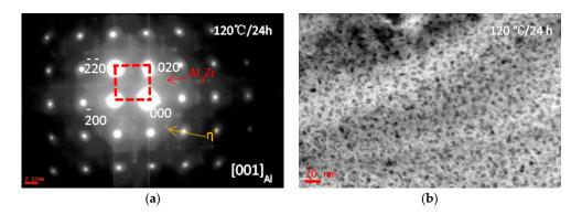
**Figure 2.** Bright-field (BF) images of the studied alloy having been solid solution treated at 470 °C for 1 h and then directly aged at 120 °C for 24 h. (a) SADP, the beam along zone axis of  $[100]_{Al}$ ; (b) bright-field image.
