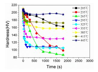
**Figure 9.** Hardness variation via the isothermal treated time on the studied samples having been solution treated at 470 °C for 1 h, isothermal heat treated for various durations, and then aged at 120 °C for 24 h.
