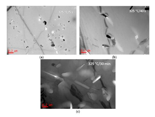
**Figure 4.** BF images of the studied alloy having been isothermal heat treated at 325 °C for different durations. The IHT durations are: (**a**) 5 s; (**b**) 40 s; and, (**c**) 30 min.
