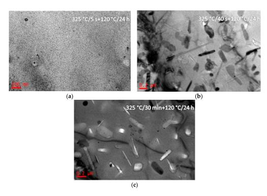
**Figure 7.** BF images of the studied alloy having been isothermal heat treated at 325 °C for different durations (5 s, 40 s, and 30 min), and then aged at 120 °C for 24 h. The isothermal heat treatment durations are: (**a**) 5 s; (**b**) 40 s; and, (**c**) 30 min.
