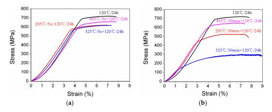
**Figure 10.** Stress-strain curves of the tensile samples having been isothermal heat treated at 205  $^{\circ}$ C, 325  $^{\circ}$ C, and 445  $^{\circ}$ C for different durations (5 s and 30 min), then aging at 120  $^{\circ}$ C for 24 h. (a) the isothermal heat treated time is 5 s; (b) the isothermal heat treated time is 30 min.
