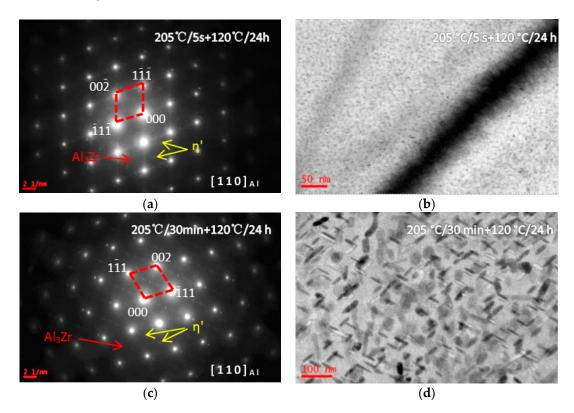
**Figure 6.** SADPs and BF images of the studied alloy having been isothermal heat treated at 205 °C for different durations (5 s and 30 min), and then aged at 120 °C for 24 h. (a) SADP from the area in (b); (b) the isothermal heat treatment is 5 s; (c) SADP from the area in (d); and (d) isothermal heat treatment is 30 min.
