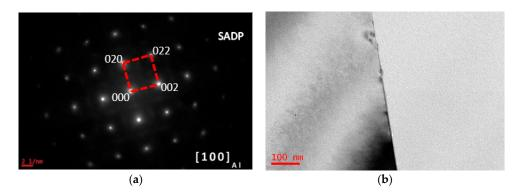
**Figure 1.** Microstructure and selected area diffraction patter (SADP) of the sample having been solution treated at 470 °C for 1 h. (a) SADP of the sample, beam along to zone axis of [100]<sub>Al</sub>; (b) bright-field image.
