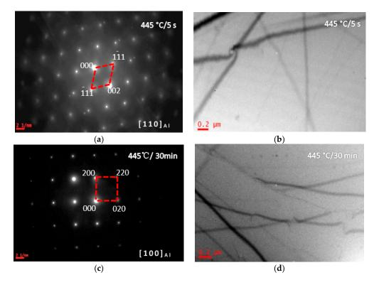
**Figure 5.** SADPs and BF images of the studied alloy having been isothermal heat treated at 445 °C for 5 s and 30 min. (a) SADP from the area in (b); (b) the isothermal heat treatment time is 5 s; (c) SADP from the area in (d); and (d) BF image, the isothermal heat treatment time is 30 min.
