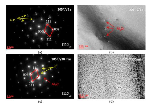
**Figure 3.** SADPs and BF images of the specimens having been isothermal heat treated at 205 °C for different durations (5 s and 30 min). (a) SADP of (b), beam along  $[110]_{AI}$ ; (b) the IHT time is 5 s; (c) SADP of (d), beam along  $[110]_{AI}$ ; and (d) the isothermal heat treatment (IHT) time is 30 min.
