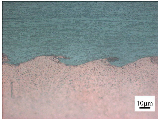
Figure 8. Optical microstructure of the etched W–Cu interface of T-6.
