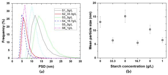
*Figure S1. Effect of starch concentration on PSD (a) and mean particles size (b), 0.01 M Cu(NO<sub>3</sub>)<sub>2</sub>/0.02 M NaBH<sub>4</sub>, flow ratio=2, flow rate=5.5 ml/s disk speed= 2400 rpm*
