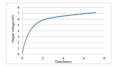
Figure 3. Turning-on drift of one accelerometer.
