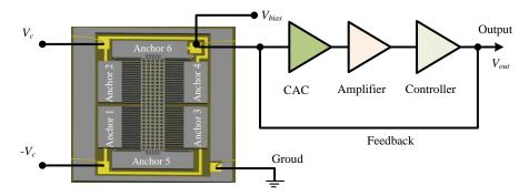
Figure 2. Sensing model of the accelerometer.
