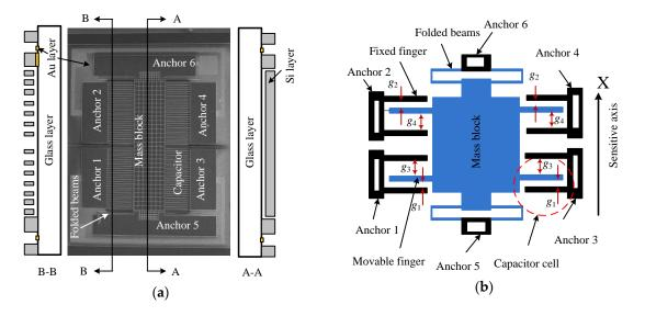
**Figure 1.** Sensor chip of the micro-accelerometer: (**a**) bi-layer structure of the micro-accelerometer; and (**b**) the simplified model of the sensor structure.
