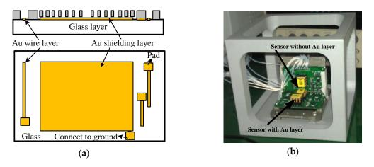
Figure 6. Shielding layer and test platform: (a) layout of shielding layer; and (b) sensors on platform.
