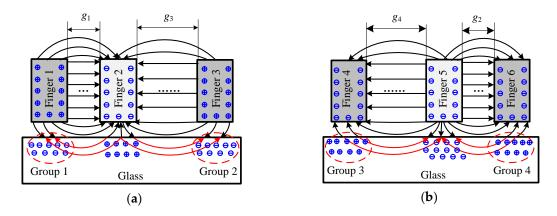
**Figure 4.** Glass polarization mechanism under an applied DC bias: (**a**) polarization of the top capacitor; and (**b**) polarization of bottom capacitor.
