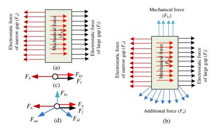
**Figure 5.** The force acting on finger: (**a**) initial state; (**b**) polarization state; (**c**) simplification of the initial state; and (**d**) simplification of the polarization state.
