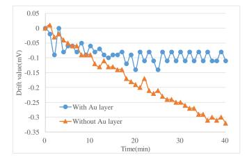
Figure 7. Comparison of sensors with and without an Au layer.
