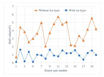
Figure 8. Reduced magnitude of drift for tested sensors with an Au layer as compared with no Au layer.
