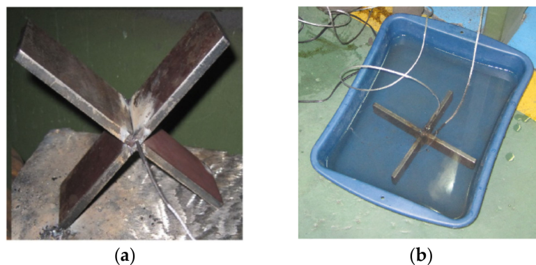
Figure 1. Connection of the thermocouples. (a) Welded specimen; (b) Connected thermocouples.
