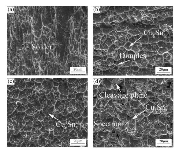
**Figure 7.** Top views of the shear fracture surfaces for the solder joints at 800-ms ultrasonic bonding times for different aging time: (**a**) 24 h; (**b**) 120 h; (**c**) 240 h and (**d**) 360 h.
