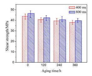
Figure 5. Shear strengths of joints after aging under different bonding times.
