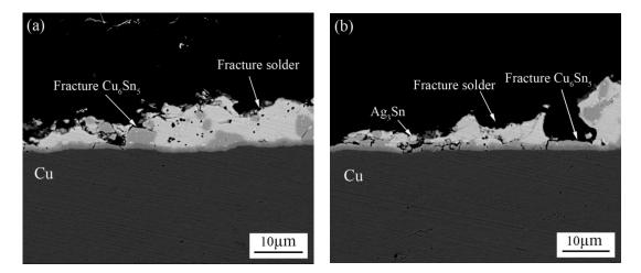
**Figure 8.** Fracture modes in solder joints formed at an 800-ms ultrasonic bonding vibration time for aging times of (**a**) 240 h and (**b**) 360 h.
