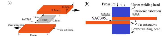
**Figure 1.** (a) Schematic of the Cu/SAC305/Cu sandwich structure and (b) the ultrasonic bonding principle.
