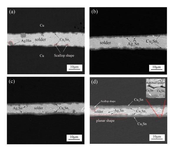
**Figure 2.** The morphologies of the cross-sectional Cu/SAC305/Cu joints formed at a 400-ms ultrasonic bonding time at different aging times of (**a**) 0 h; (**b**) 120 h; (**c**) 240 h and (**d**) 360 h. The inset in (d): the local enlargement image at the interfaces.
