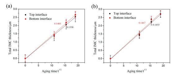
**Figure 4.** The total  $Cu_6Sn_5$  and  $Cu_3Sn$  thickness of the top and bottom interfaces with aging time at different bonding times: (a) 400 ms and (b) 800 ms.
