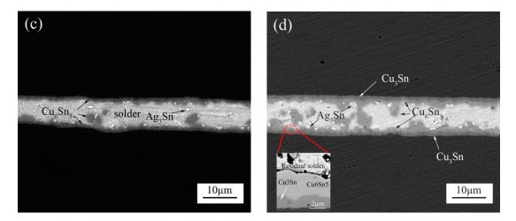
**Figure 3.** The morphologies of the cross-sectional Cu/SAC305/Cu joints formed at an 800-ms ultrasonic bonding time at different aging times of (**a**) 0 h; (**b**) 120 h; (**c**) 240 h and (**d**) 360 h. The inset in (d): the local enlargement image at the interfaces.
