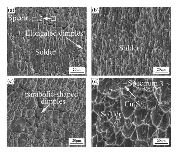
**Figure 6.** Top views of the shear fracture surfaces for the solder joints at a 400-ms ultrasonic bonding time for different aging times: (**a**) 24 h; (**b**) 120 h; (**c**) 240 h and (**d**) 360 h.
