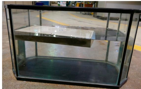
**Figure 5.** FLCC specimen floating in a water tank.
