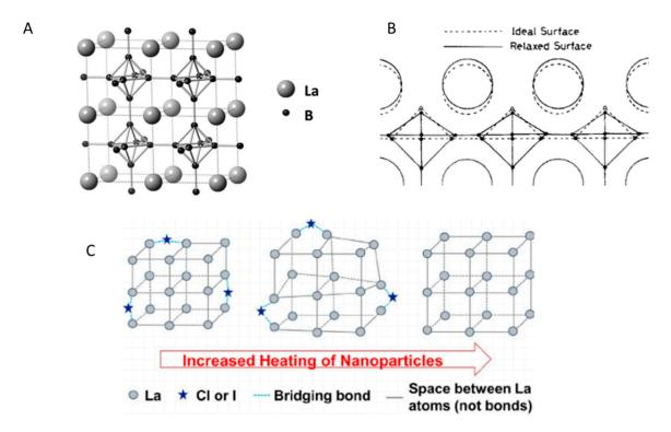
**Figure 2.** (**A**) Four unit cells of lanthanum hexaboride (LaB<sub>6</sub>) with a lattice constant of approximately 4.15 Å (reprinted from [48]). (**B**) Position of La (circle) and B<sub>6</sub> (diamond) in relaxed and ideal states on LaB<sub>6</sub> surface (reprinted from [49]). (**C**) Removal of halogen bridge between La atoms with continued heating of LaB<sub>6</sub> nanoparticle (reprinted from [58]).
