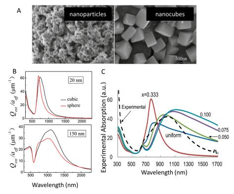
**Figure 6.** (**A**) SEM images of LaB<sub>6</sub> nanoparticles and nanocubes (reprinted from [57]). (**B**) Comparison of extinction efficiencies divided by effective radius between cubic and spherical LaB<sub>6</sub> particles (reprinted from [82]). (**C**) Absorption cross sections calculated for 100,000 LaB<sub>6</sub> oblate particles with different aspect ratios and a standard deviation of 0.1 (reprinted from [81]).
