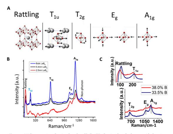
**Figure 3.** (**A**) Raman active vibrational modes of LaB<sub>6</sub>; (**B**) vibrational mode changes with changing nanoparticle sizes; and (**C**) shifting vibrational modes of 6.2 nm particles with varying B content (reprinted from [63]).
