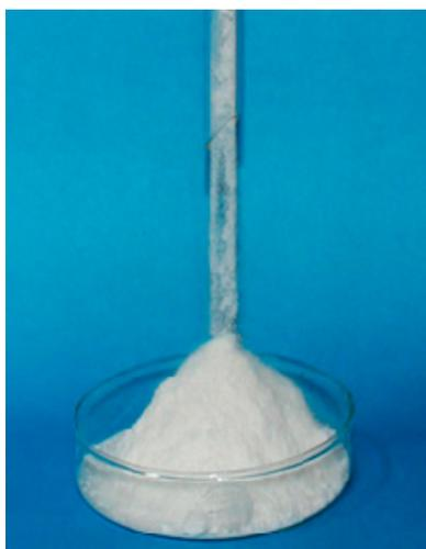
**Figure 2.** Free-flowing HSCP-70 from a glass funnel.
