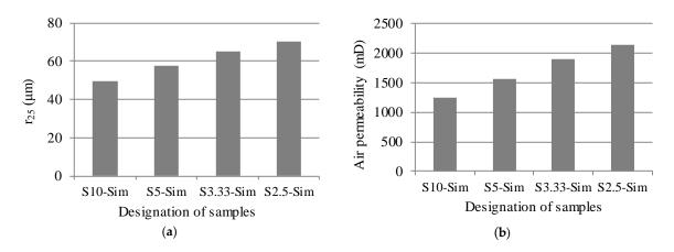
**Figure 15.** Calculation of air permeability of the samples with different sizes. (**a**) Pore throat radius corresponding to the 25th percentile of saturation of mercury. (**b**) Calculated permeability of the samples. The air permeability was calculated from the porosity and the pore throat radius according to Equation (4).
