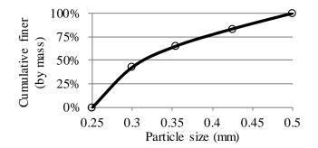
**Figure 1.** Particle size distribution of the quartz sand used for the preparation of artificial sandstone, as determined by sieving.
