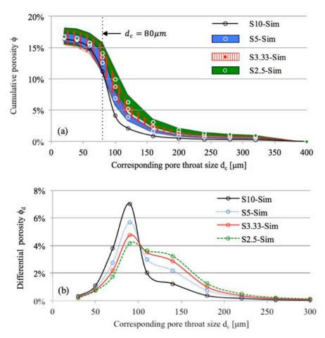
**Figure 10.** Pore throat size of artificial sandstone samples with different sizes determined by MIP simulation. (a) Cumulative porosity. The cumulative porosity curves of smaller samples (S5-Sim, S3.33-Sim and S2.5-Sim) are shown in shaded area, indicating standard deviation of the simulated results. (b) Differential porosity. The differential porosity curves of the small samples are calculated from the average values of the cumulative porosity.
