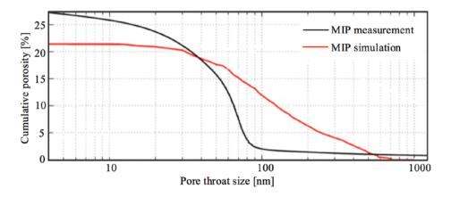
**Figure 14.** Comparison of PSD curves of a cement paste (OPC CEM I 42.5, water-to-cement ratio (w/c) 0.35, after 28 days of hydration) determined by MIP measurement and MIP simulation [25].
