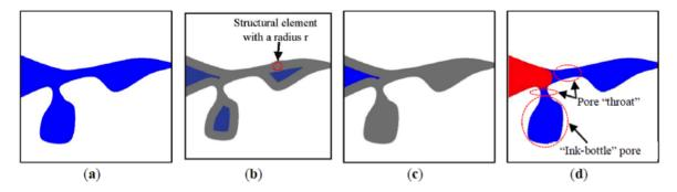
**Figure 7.** Two-dimensional illustration of steps for simulating mercury intrusion into porous material; solid is shown in white, pore in blue, and mercury in red. (**a**) original porous system, (**b**) pore space after erosion by a structural element, (**c**) pore space connected to the surfaces of material, (**d**) pore space after dilation; area in red represents mercury-intruded pore space.
