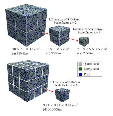
**Figure 5.** Digital microstructure of sandstone samples with different sizes (digital resolution =  $10 \,\mu$ m/voxel). Quartz sand is shown in grey, epoxy resin in green, and pores in blue. The size of the large sample (S10-Sim) is taken as a reference. The lengths of small samples (i.e., S5-Sim, S3.33-Sim, and S2.5-Sim) are scaled down by a factor *n* = 2, 3, and 4, respectively.
