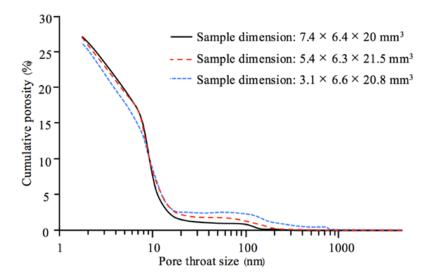
**Figure 13.** Comparison of the pore throat size distribution (PSD) curves of cement pastes (water-to-cement ratio = 0.5, cured in water for 2 years) with different dimensions. The PSD curves were determined by MIP measurement [17].
