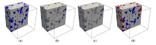
**Figure 8.** Illustration of steps for simulating mercury intrusion into digital microstructure of S2.5-Sim ( $d_c = 120 \ \mu m$ ), solid is shown in light grey, pore in blue, and mercury in red. (**a**) original porous system, (**b**) pore space after erosion by a structural element, (**c**) pore space connected to the surfaces of the material, (**d**) pore space after dilation; area in red represents mercury-intruded pore space.
