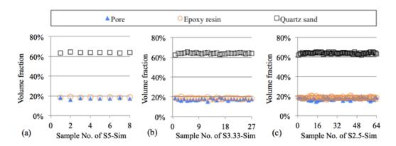
**Figure 6.** Volume fraction of pore, epoxy resin, and quartz sand in digital microstructures of sandstone samples with different sizes. (**a**) S5-Sim (8 samples), (**b**) S3.33-Sim (27 samples), (**c**) S2.5-Sim (64 samples).
