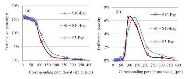
**Figure 9.** (a) Cumulative porosity and (b) differential porosity of artificial sandstone samples with different sizes as determined by laboratory MIP measurements.
