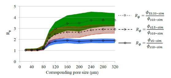
**Figure 12.** Effect of sample size on the cumulative porosity of mercury-intruded pores.  $R_s$  is the ratio of the cumulative porosity of small sample (S5-Sim, S3.33-Sim, or S2.5-Sim) to that of large sample (S10-Sim). The shaded areas indicate standard deviations of the simulated results.
