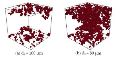
**Figure 11.** Percolation analysis of mercury-intruded pores in sandstone sample (S5-Sim). Mercury (in red) is intruded from the top and bottom surfaces of the sample. (a) The mercury has only penetrated the outer part (adjacent to the top and bottom surfaces) of the sample when  $d_c = 100 \mu m$ . (b) The mercury-intruded pores have percolated in the sample when  $d_c = 80 \mu m$ .
