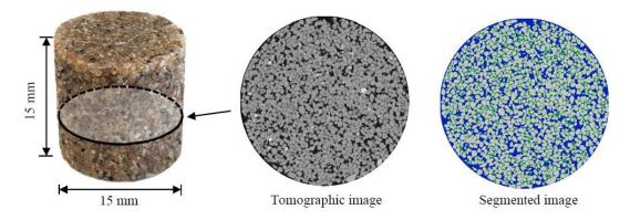
**Figure 4.** Sandstone sample prepared for CT scan test. The sandstone was made of quartz sand and epoxy resin, and had a bulk density of  $2130 \text{ kg/m}^3$ . In the segmented image, quartz sand is shown in grey, epoxy resin in green, and pores in blue.
