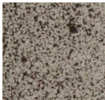
Figure 3. An example of a random speckle pattern.
