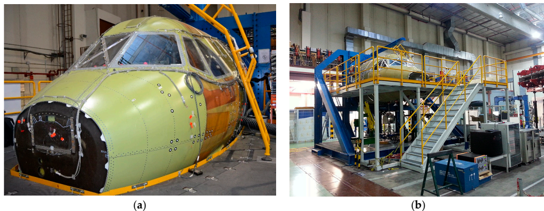
Figure 1. Clean Sky/Green Regional Aircraft MT2 cockpit demonstrator (a) and test rig (b) developed by Airbus Defence and Space.
