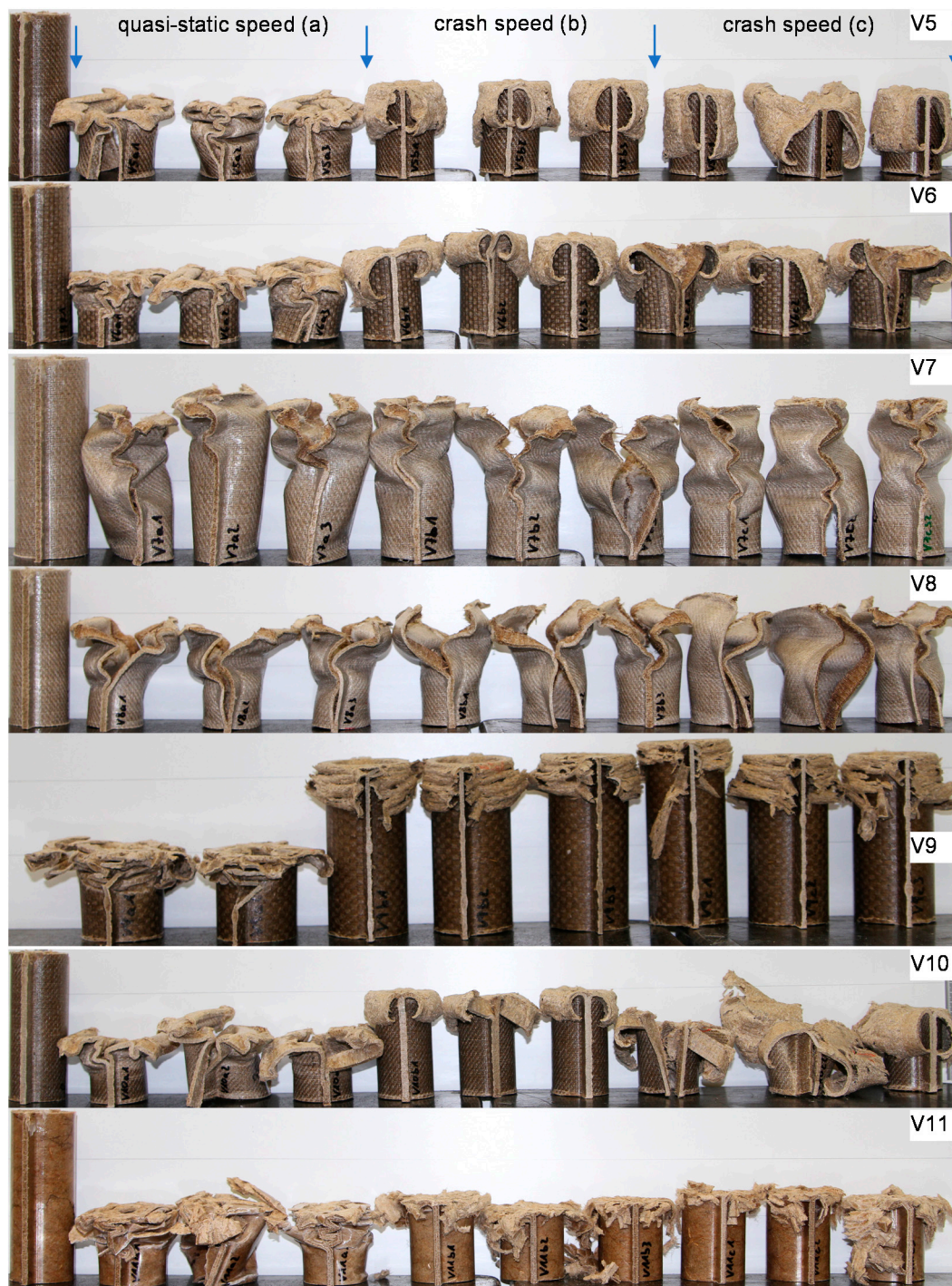
Figure 4. Deformed specimens of test series V5–V11. Left: undeformed specimen; middle: specimens tested at quasi-static speed; right: specimens tested at crash speed.
