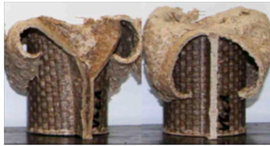
Figure 15. Rear and front part of V6_c specimen after crash test.
