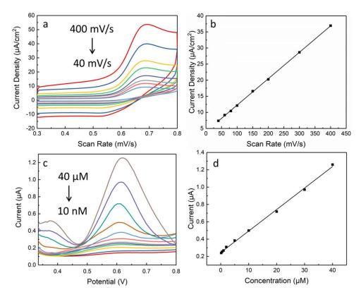
**Figure 3.** (a) CV responses of AuNP/graphene electrodes after 4-min electrodeposition in 50 μM vanillin/PBS buffer with various scan rates and (b) the corresponding current density of oxidation peak. (c) DPV curves of AuNP/graphene electrodes with different vanillin concentrations and (d) the linear dynamic detection range.
