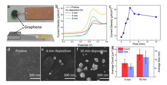
**Figure 2.** (a) Photograph of as-prepared graphene-diamond hybrid electrode. (b) CV responses of the electrodes with different deposition periods of AuNPs in PBS containing 50  $\mu$ M vanillin (scan rate: 100 mV/s). (c) The changes of peak current density of prepared electrodes with different deposition periods. SEM images of (d) pristine graphene and AuNP/graphene after (e) 4 and (f) 16 min of electrodeposition. (g) The average count and size of AuNPs.
