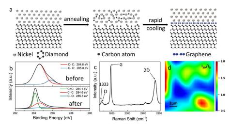
**Figure 1.** (**a**) Schematic illustration of the conversion process of the graphene–diamond hybrid through catalytic thermal treatment. (**b**) XPS C1s spectrum of pristine HPHT diamond before and after sp<sup>3</sup>-to-sp<sup>2</sup> conversion. (**c**) A typical Raman spectrum and (**d**) Raman mapping of graphene films formed on the diamond surface.
