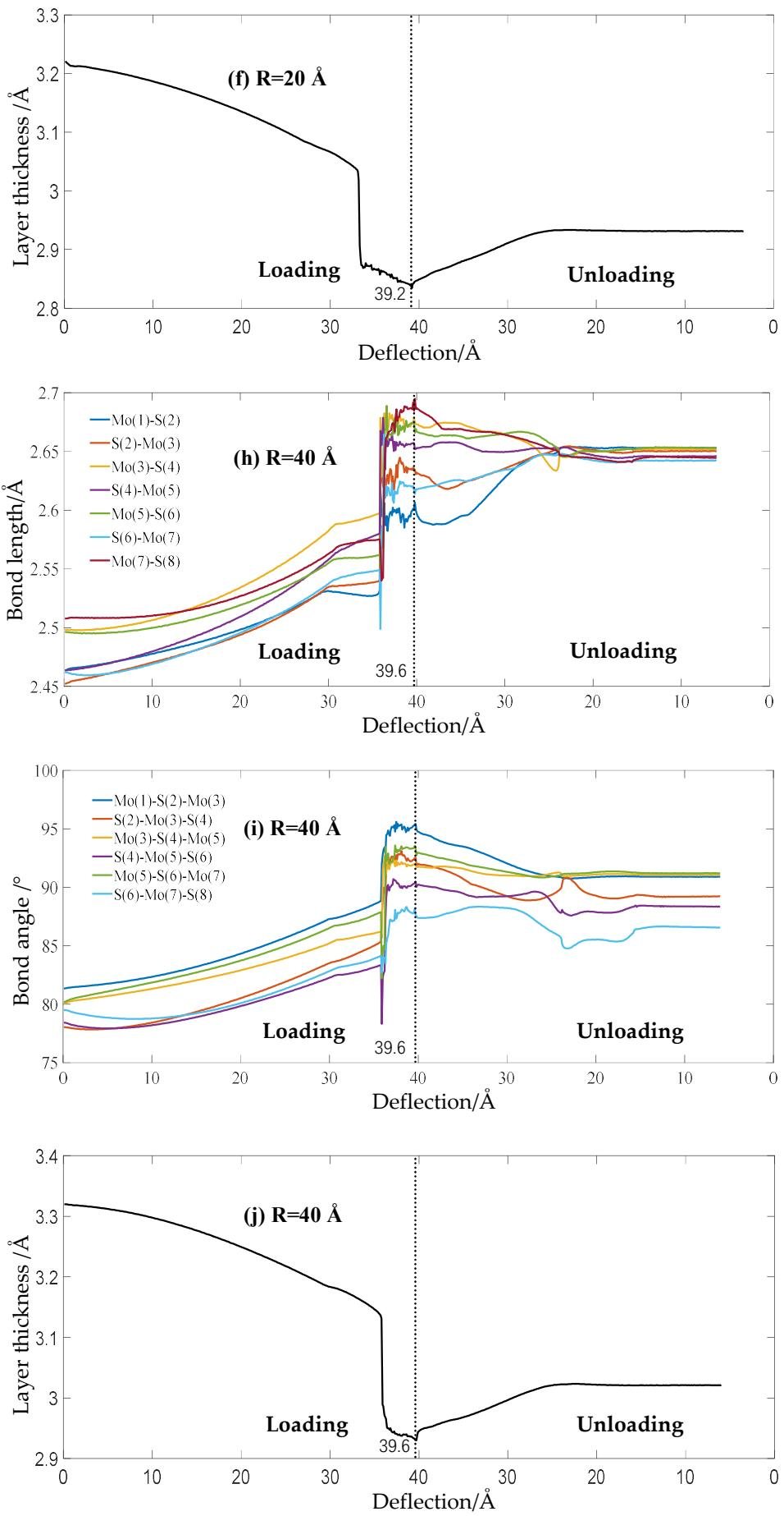
**Figure 1.** The Mo-S and S-Mo bond lengths (a, d and h), S-Mo-S bond angles and Mo-S-Mo angles (b, e and i), and layer thickness of S-S (c, f and j) versus deflection during the loading process and unloading process with indenter radii of 15 Å, 20 Å and 40 Å (The labeled atoms are shown in Figure 3.).
