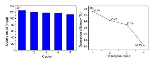
**Figure 12.** (a) Regeneration studies of g-PAM/OVerm after five cycles; and (b) evolution of the desorption efficiencies during four-time desorption.
