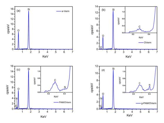
**Figure 6.** Energy dispersive spectrometer (EDS) patterns of (**a**) a-Verm; (**b**) OVerm; (**c**) PAM/OVerm; (**d**) g-PAM/OVerm.
