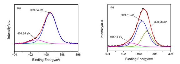
Figure 15. XPS N 1s spectra of g-PAM/OVerm: (a) before Pb(II) adsorption and (b) after Pb(II) adsorption.
