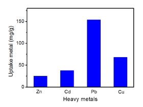
**Figure 11.** Effect of the presence of competitor ions on adsorption of Pb(II) (Reaction conditions: contact time t = 120 min, pH = 5.5, T = 30  $^{\circ}$ C).
