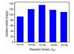
**Figure 3.** Effect of the grafting reaction times on Pb(II) removal and  $q_e$ . (Reaction conditions:  $C_i = 400 \text{ mg} \cdot \text{L}^{-1}$ , pH = 8, T = 50 °C.)
