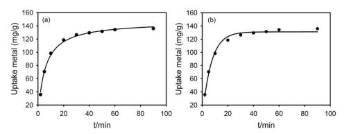
**Figure 13.** (a) The pseudo-second-order kinetic model, (b) the pseudo-first-order kinetic model for the adsorption of Pb(II) by g-PAM/OVerm (Reaction conditions: initial suspension pH = 5.5, 0.05 g g-PAM/OVerm, T =  $30 \degree$ C).
