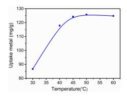
**Figure 2.** Effect of temperature of the grafting reaction on Pb(II) removal and  $q_e$ . (Reaction conditions:  $C_i = 400 \text{ mg} \cdot \text{L}^{-1}$ , pH = 8, grafting reaction times  $t_1 = 1 \text{ h}$ ,  $t_2 = 1 \text{ h}$ .)
