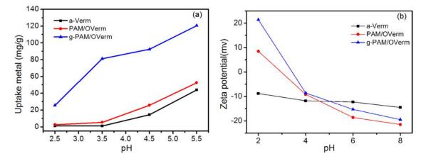
**Figure 10.** (a) Effect of pH on adsorption of Pb(II) (Reaction conditions:  $C_i = 400 \text{ mg} \cdot \text{L}^{-1}$ , contact time t = 120 min, 0.05 g adsorbent); and (b) effect of solution pH on the zeta potential of a-Verm, PAM/OVerm and g-PAM/OVerm.
