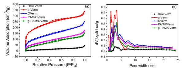
**Figure 9.** (a) N<sub>2</sub> adsorption–desorption isotherms and (b) pore width distribution of Raw Verm, a-Verm, OVerm, PAM/OVerm and g-PAM/OVerm.
