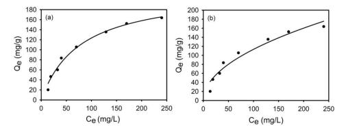
**Figure 14.** (a) Langmuir plot and (b) Freundlich plot for the adsorption of Pb(II) by g-PAM/OVerm (Reaction conditions: initial suspension pH = 5.5, 0.05 g g-PAM/OVerm, T = 30 °C).
