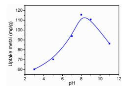
**Figure 1.** Effect of the pH of the grafting reaction on Pb(II) removal and  $q_e$ . (Reaction conditions:  $C_i = 400 \text{ mg} \cdot \text{L}^{-1}$ , T = 50 °C, grafting reaction times  $t_1 = 1 \text{ h}$ ,  $t_2 = 1 \text{ h}$ )
