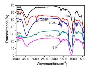
**Figure 4.** Fourier transform infrared (FTIR) spectra of (a) raw vermiculite (Verm), (b) acid-activated vermiculite (a-Verm), (c) 3-(triethoxysilyl)propyl methacrylate-modified acid vermiculites (OVerm), (d) polyacrylamide (PAM)/OVerm and (e) triethylenetetramine-grafted polyacrylamide (g-PAM)/OVerm.
