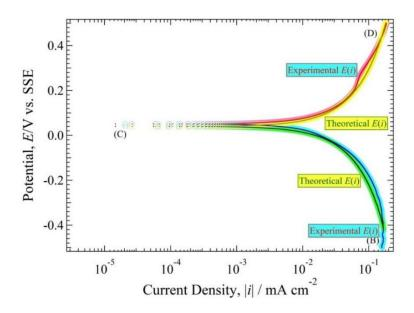
**Figure 13.** Superimposition of the experimental polarization curve and theoretical polarization curve obtained by solving the polarization resistance equation.
