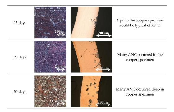
Figure 1. Surface and cross-section observations of Cu tube specimen immersed in 10<sup>3</sup> ppm Cu(HCOO)<sub>2</sub>.
