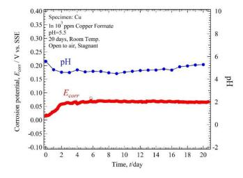
**Figure 6.** Corrosion potential, solution pH and time plot of Cu tube specimen in  $10^3$  ppm Cu(HCOO)<sub>2</sub> solution with solution pH 5.5.
