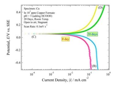
**Figure 9.** Polarization curve of Cu tube specimen in  $10^3$  ppm Cu(HCOO)<sub>2</sub> solution at the immersion period of 0 days and 20 days with solution pH 3.
