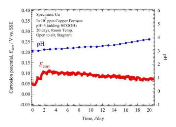
**Figure 7.** Corrosion potential, solution pH and time plot of Cu tube specimen in  $10^3$  ppm Cu(HCOO)<sub>2</sub> solution with solution pH 3.
