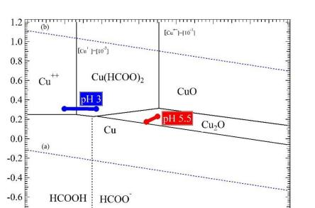
**Figure 12.** *E*-pH Diagram of Cu and Cu(HCOO)<sub>2</sub> with pH condition 5.5, with the assumption that the concentration of total dissolved copper ions  $[Cu^{++}]$  was  $10^{-3}$  mol kg<sup>-1</sup>.
