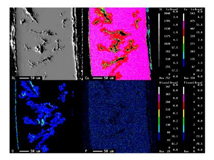
**Figure 5.** The result of SEM image of the copper tube after being immersed 30 days in  $10^3$  ppm Cu(HCOO)<sub>2</sub>; EPMA led to corresponding elements of copper, oxygen, and phosphorus.
