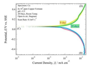
**Figure 8.** Polarization curve of Cu tube specimen in  $10^3$  ppm Cu(HCOO)<sub>2</sub> solution at the immersion period of 0 days and 20 days with solution pH 5.5.
