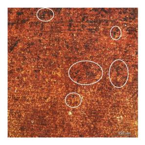
**Figure 2.** Surface observations of Cu tube specimen immersed in  $10^3$  ppm Cu(HCOO)<sub>2</sub> after 10 days immersion.
