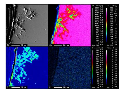
**Figure 4.** The result of scanning electron microscope (SEM) image of the copper tube after being immersed 15 days in 10<sup>3</sup> ppm Cu(HCOO)<sub>2</sub>; electron probe micro-analysis (EPMA) led to corresponding elements of copper, oxygen, and phosphorus.
