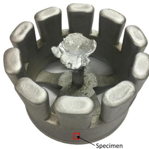
Figure 12. The casting obtained from the 3D-printed sand mold.
