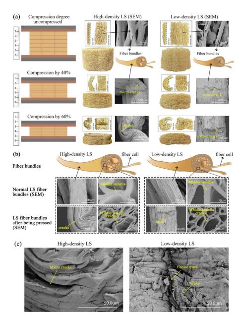
**Figure 5.** The morphology of the two types of LS columns and their fiber bundles: (**a**) the surface morphology of LS columns compressed to different degrees and the micro morphology of their inner fiber bundles, (**b**) the morphology of a fiber cell section before and after the compression of LS columns and (**c**) the surface morphology of HD and LD LS columns.
