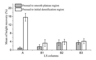
**Figure 7.** Mean of height recovery of LS columns. (A refers to LD LS columns with densities ranging from 15 to 35 kg/m<sup>3</sup>; B1, B2, and B3 refer to HD LS columns with densities ranging from 15 to 35 kg/m<sup>3</sup>, 41 to  $50 \text{ kg/m}^3$ , and 50 to  $65 \text{ kg/m}^3$ , respectively.
