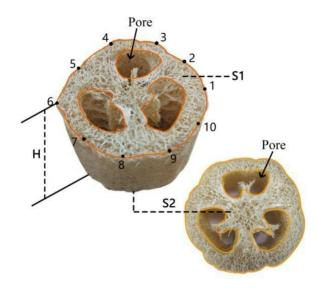
Figure 2. The method for testing the volume of luffa sponge column.
