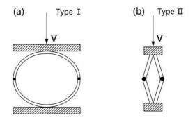
Figure 6. Two simple types of energy-absorbing structure.
