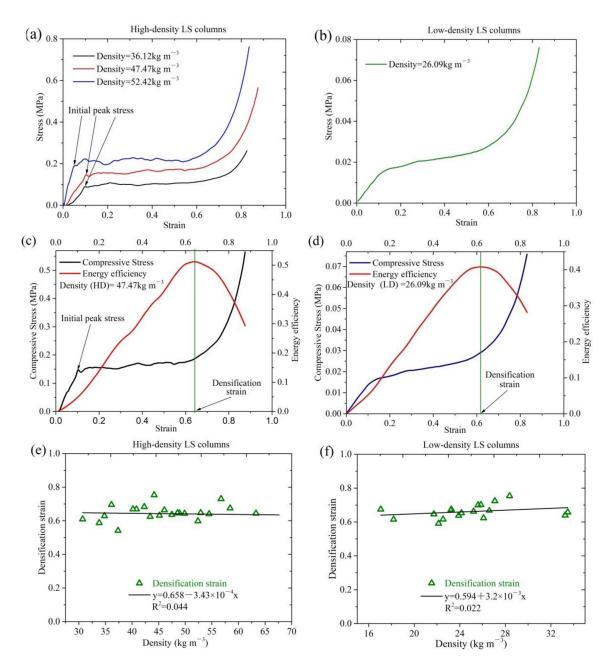
**Figure 3.** The mechanical properties of the two types of LS column: (a) the stress–strain curves of high-density LS columns, (b) the stress–strain curve of low-density LS columns; (c,d) illustration of the densification strain method; (e) densification strain of high-density LS columns; and (f) densification strain of low-density LS columns.
