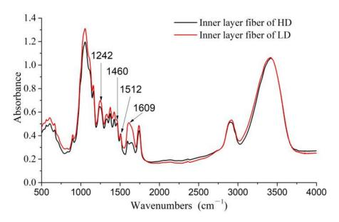
Figure 4. Fourier transform infrared (FTIR) spectra of high/low-density LS fibers.
