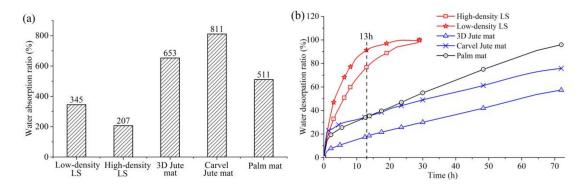
**Figure 8.** (a) Water absorption of five types of plant mattress filling materials, (b) water desorption of five types of plant mattress filling materials.
