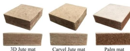
**Figure 9.** The three types of plant fiber mats.
