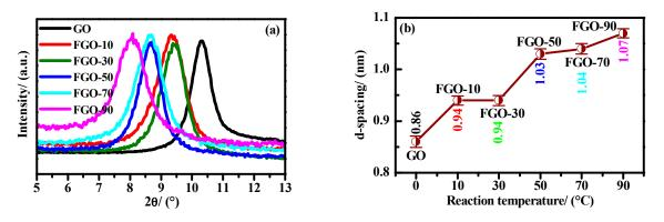
Figure 1. XRD patterns (a) and d-spacing (b) of GO and FGO-T samples.
