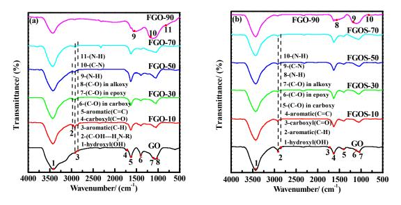
Figure 4. FT-IR spectra of GO and FGO-T samples: (a) without and (b) with methanol soaking.
