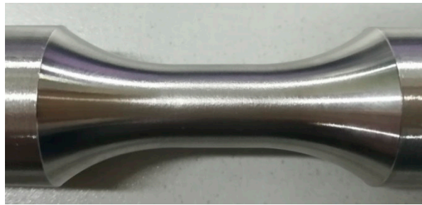
Figure 7. Specimen under -10\% compressive strain.
