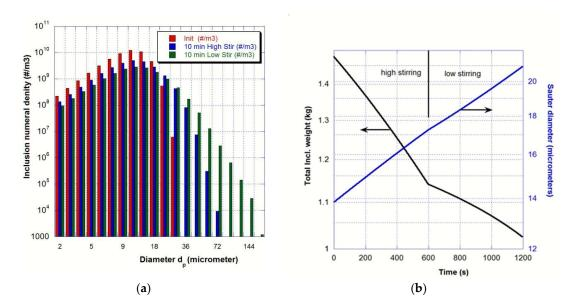
**Figure 6.** Average values of the non-metallic inclusion population in the ladle (**a**) PSD at three different times (initial in red, after 10 min of high stir in blue, and after 10 min low stir in green) (**b**) Time evolution of the total weight of non-metallic inclusions and of Sauter diameter.
