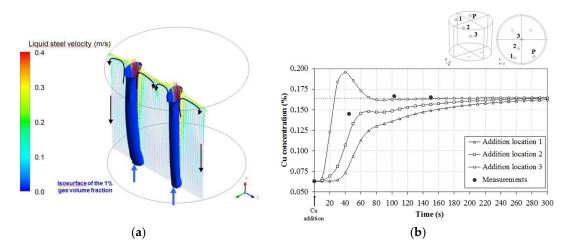
**Figure 5.** Hydrodynamic simulation of a 60 t steel ladle. (a) Predicted velocity of the liquid steel along with the argon plumes (isosurface of the 1% gas volume fraction) in a vertical plane passing through the porous plugs for a weak aeration. (b) Calculated Cu concentration profiles at the P sampling point compared with plant measurements for three platelet addition locations in the 60 t gas-stirred ladle.
