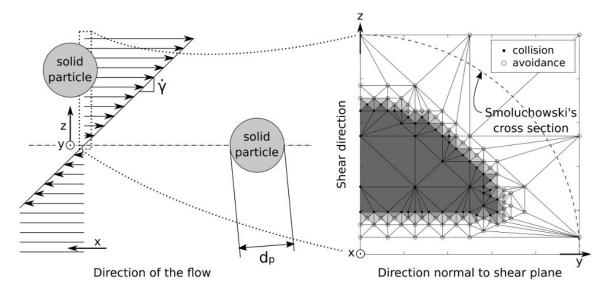
Figure 2. Simulation setup and example cross section derivation from 363 simulations of two identical spherical particles at  $\text{Re}_{\gamma} = 0.213$ .
