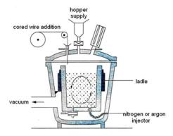
Figure 1. Schematic of a gas-stirred ladle.
