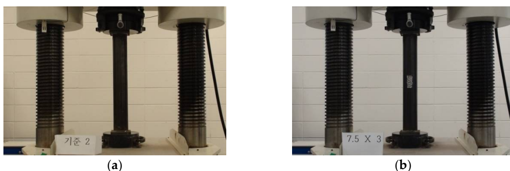
Figure 2. Experimental setup of compressive loading test specimen: (a) CR-H0W0-2 specimen; and (b) CR-H7.5W3 specimen.
