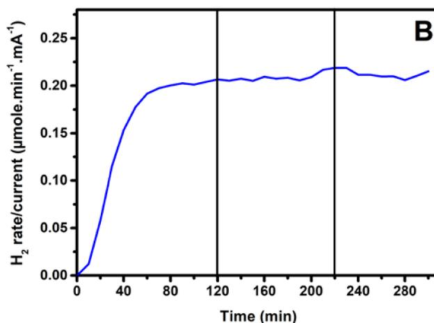
**Figure 5.** (A) Hydrogen production rates recorded by using the same photoanode and three different counter electrodes: (1) carbon paper without electrocatalyst; (2) carbon paper and RGO; and (3) carbon paper and carbon black + Pt. (B) Plot of the hydrogen production rate (3) divided by the corresponding current. The vertical lines show the times when the applied bias was changed: 0.5 V → 1.0 V → 1.5 V vs. RHE.
