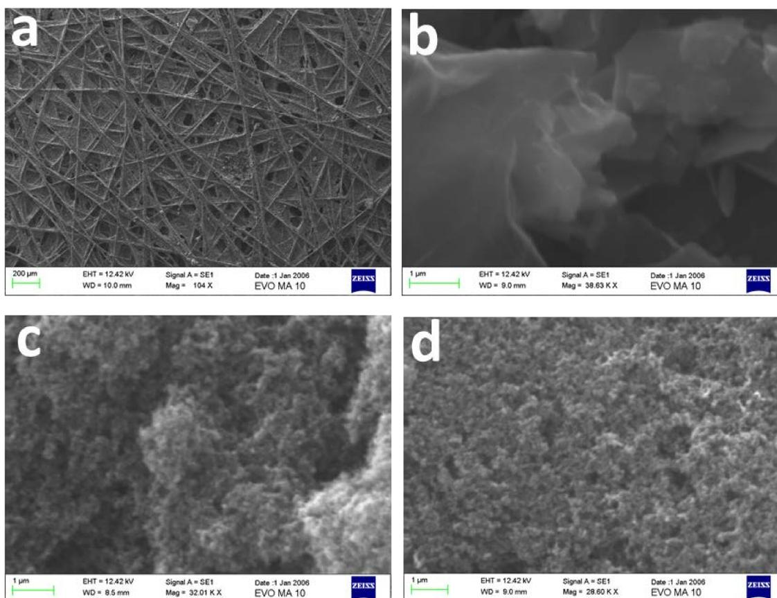
**Figure 3.** SEM images of the carbon paper used in this work: (a) plain and (b–d) covered with various electrocatalysts: (b) reduced graphene oxide (RGO); (c) carbon black; and (d) carbon black and Pt. The scale bar is 200  $\mu\text{m}$  in (a) and 1  $\mu\text{m}$  in (b–d).
