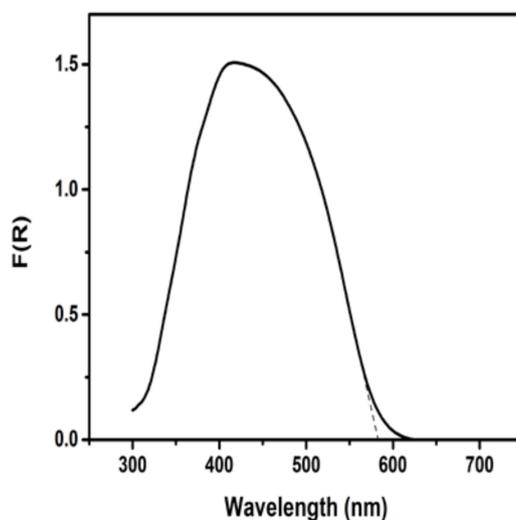
**Figure 2.** Diffuse reflectance absorption spectrum of the combined CdS/ $\text{TiO}_2$  photocatalyst film.
