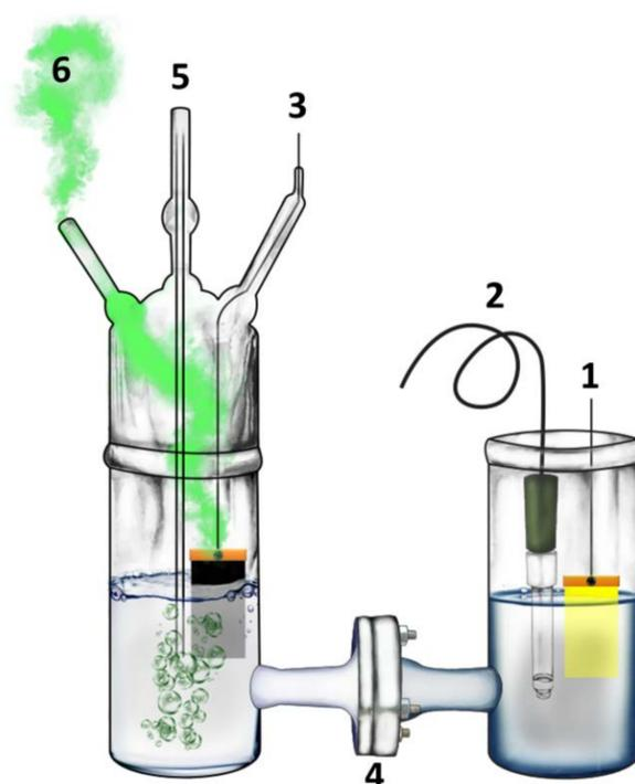
**Figure 1.** Graphical design of the employed reactor: (1) photoanode; (2) reference electrode; (3) counter electrode; (4) ion transfer membrane; (5) tube for the introduction of Ar; and (6) exhaust of Ar mixed with H<sub>2</sub>.
