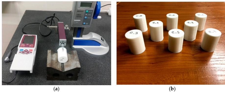
**Figure 2.** (a) Surface roughness measurement setup (b) Printed samples for experiment 1.
