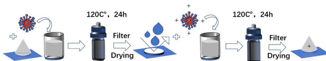
**Figure 1.** Main process steps for preparing antistatic, oil-cleaning, shell-based materials.
