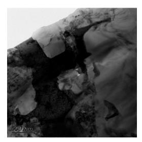
Figure 8. Bright field TEM micrograph of the Al<sub>2</sub>O<sub>3</sub>/30glass/30Cu<sub>f</sub> composite.
