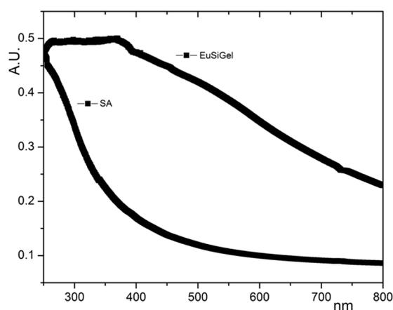
**Figure 3.** UV–vis absorbance spectra of EuSiGel and reference SA.
