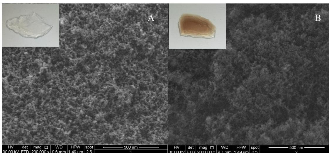
**Figure 4.** SEM images of (A) reference SA and (B) EuSiGel. Pictures of the corresponding samples are also reported (upper-left corner).
