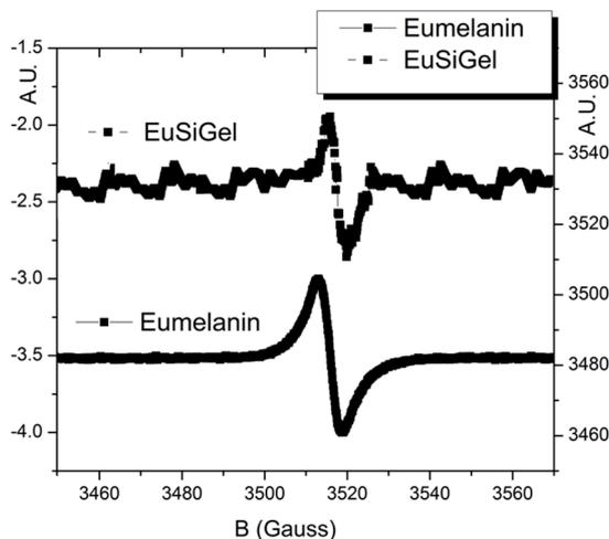
**Figure 2.** Electron Paramagnetic Resonance (EPR) spectra of the EuSiGel (top line) and reference eumelanin (bottom line).
