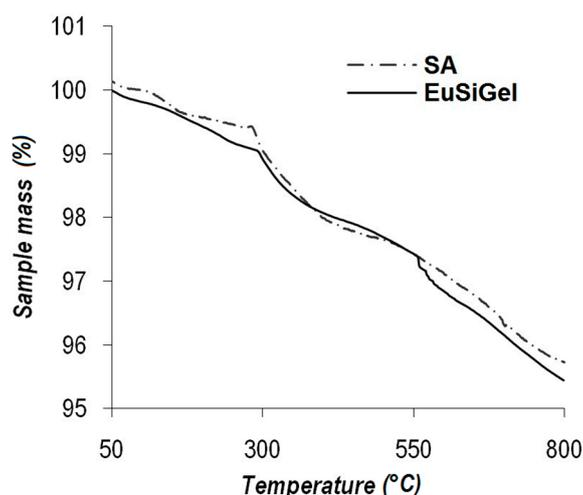
**Figure 1.** Thermogravimetric analysis of the parent silica aerogel (SA) and the eumelanin-coated hybrid (EuSiGel) in an oxidative environment (air).
