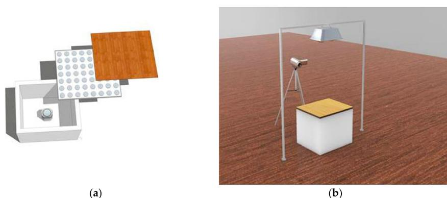
**Figure 2.** Schematic diagram of testing of thermo-regulated performance: (a) room model; (b) testing system.
