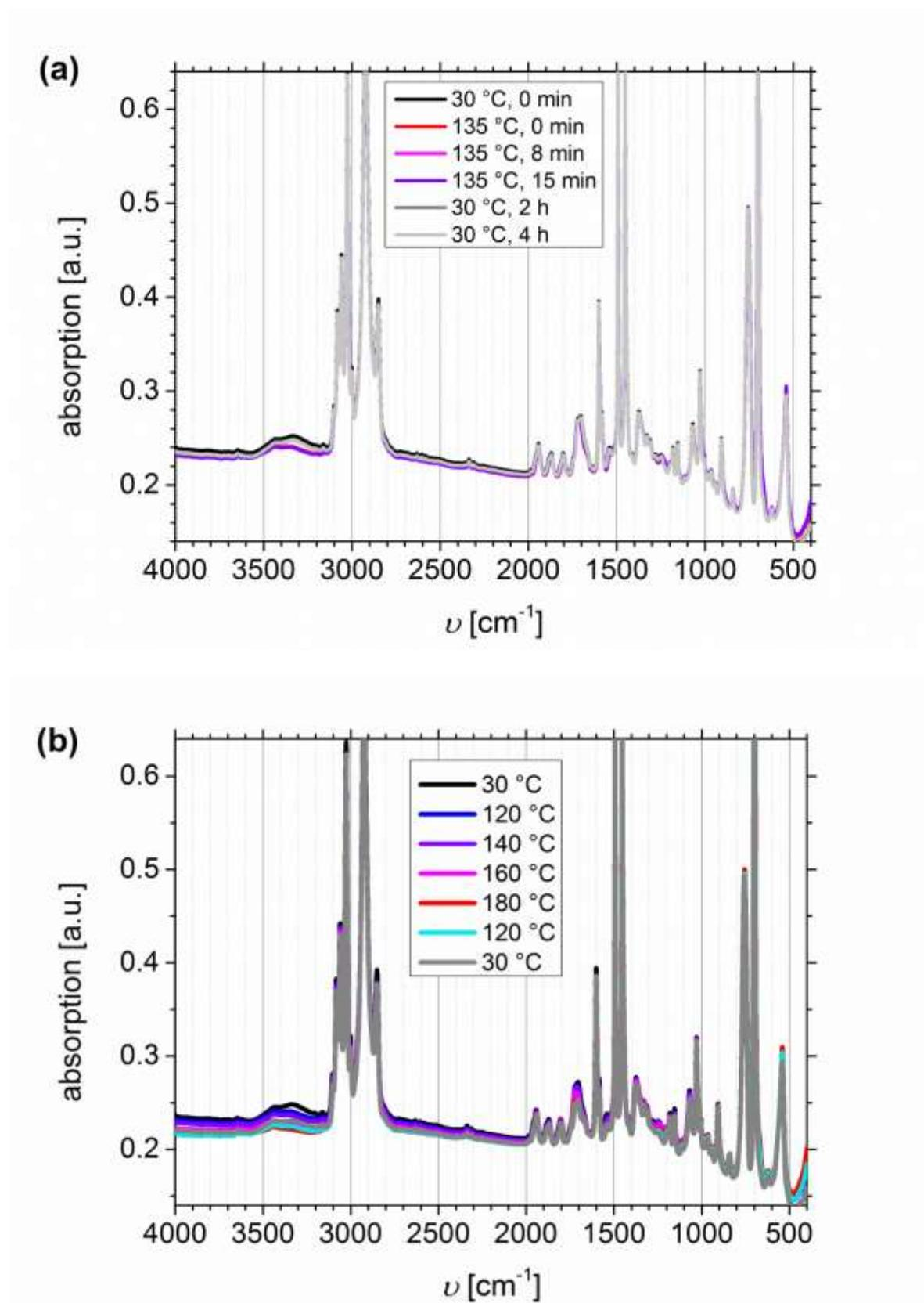
**Figure S1:** Full range temperature dependent FTIR spectra of I<sub>1.5</sub>S<sub>96.1</sub>L<sub>2.4</sub><sup>82</sup>-DETA with  $D_i = 48\%$  with a “DMA related” temperature profile: (a) related to melt pressing, and (b) related to oscillatory shear experiment with 1 h controlled holding of temperature.
