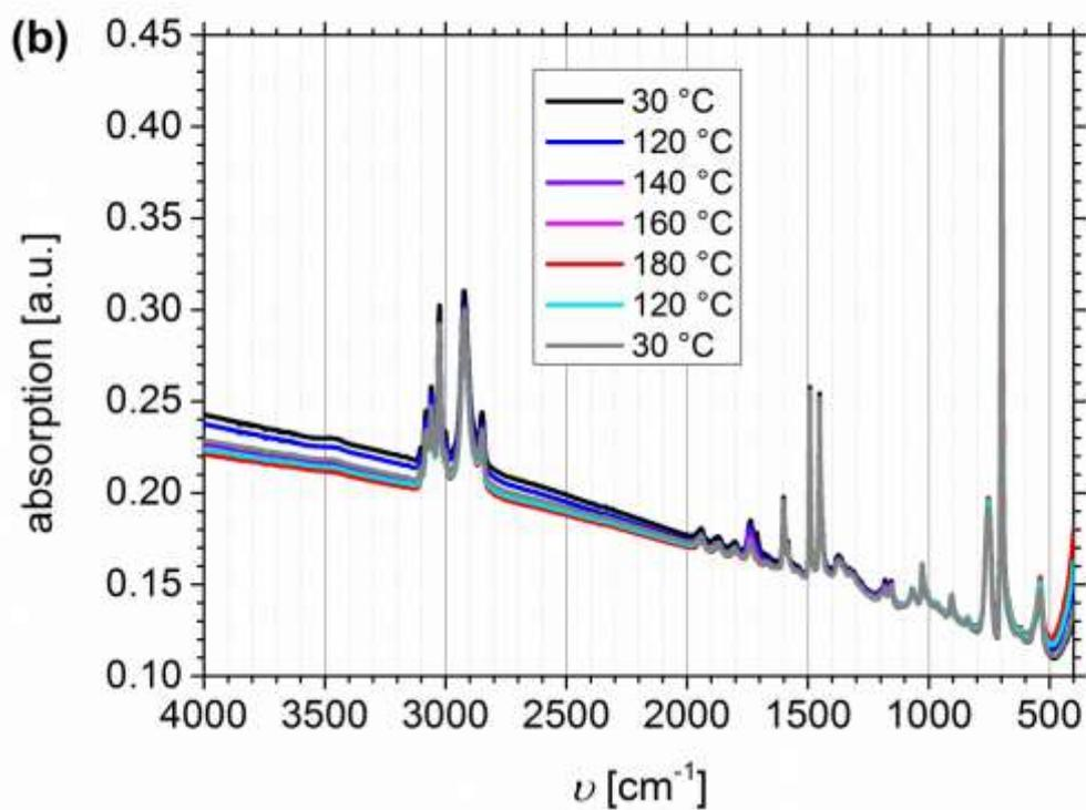
**Figure S2:** Full range temperature dependent FTIR spectra of  $I_{1.5}S_{96.1}I_{2.4}^{82}$ -SA with  $D_i = 33\%$  with a “DMA related” temperature profile: (a) related to melt pressing, and (b) related to oscillatory shear experiment with 1 h controlled holding of temperature.
