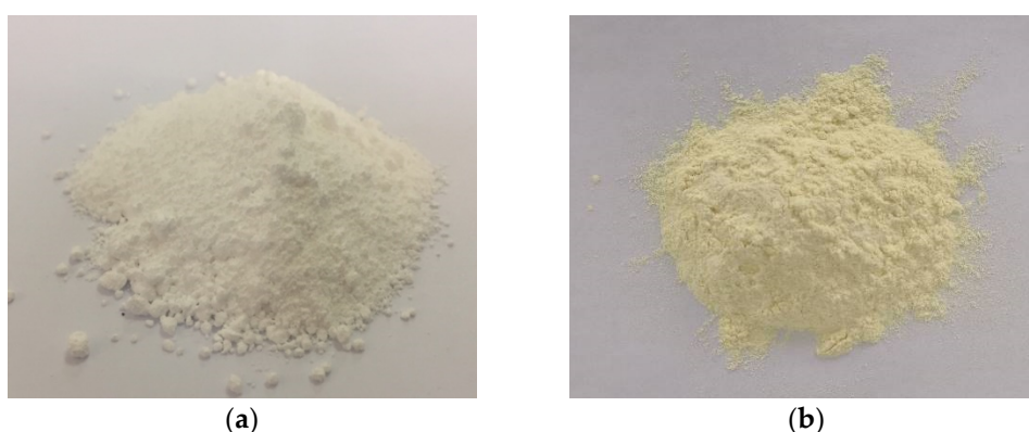
Figure 2. The original nano-TiO 2 and modified nano-TiO 2 . (a) Original TiO 2 and (b) Modified TiO 2 .
