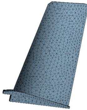
Figure 3. Finite element model of turbine blade.
