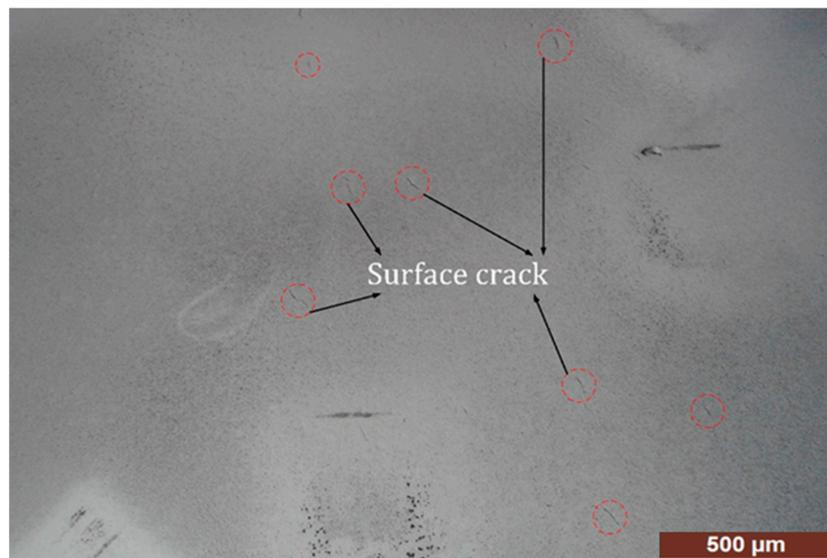
**Figure 8.** Surface cracks after performing magnetic particle testing.
