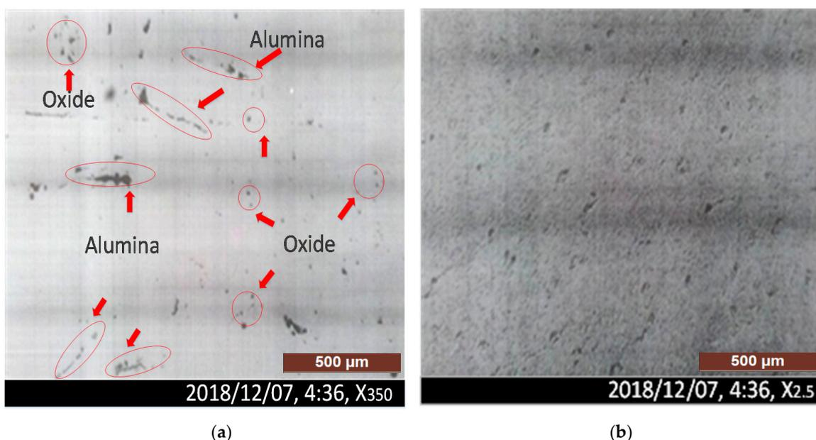
**Figure 11.** (a) Micro-inclusions, oxide and alumina-type inclusions, observed as per ASTM E-45 (b) The specimen was hotly etched in HCl (1:1), as inclusions were observed and randomly distributed as per ASTM E-381. The random condition is R-5.
