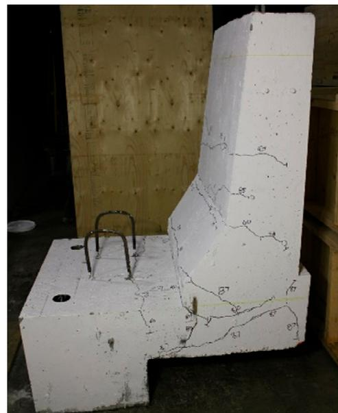
(b) Crack pattern at failure
