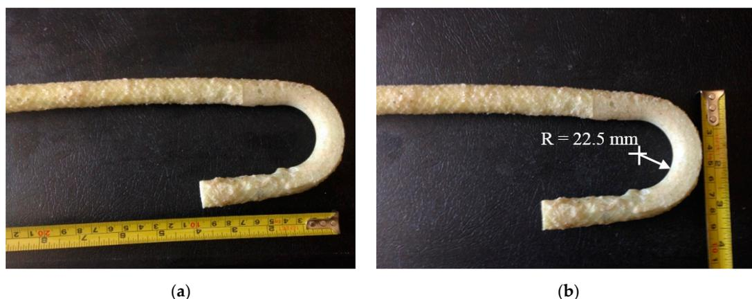
**Figure 2.** Views of the developed GFRP bar with 180° hook. (a) length of the hook; (b) radius of the hook.
