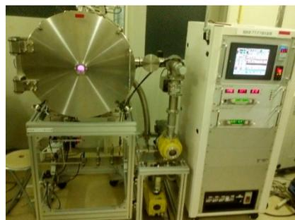
Figure 4. Appearance of the plasma nitriding machine.
