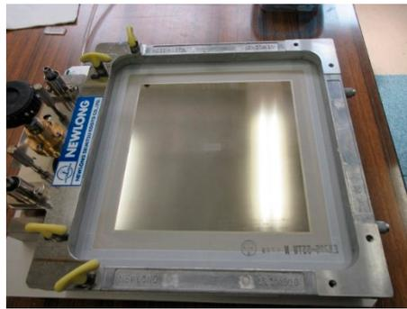
Figure 2. Appearance of screen-printing system.
