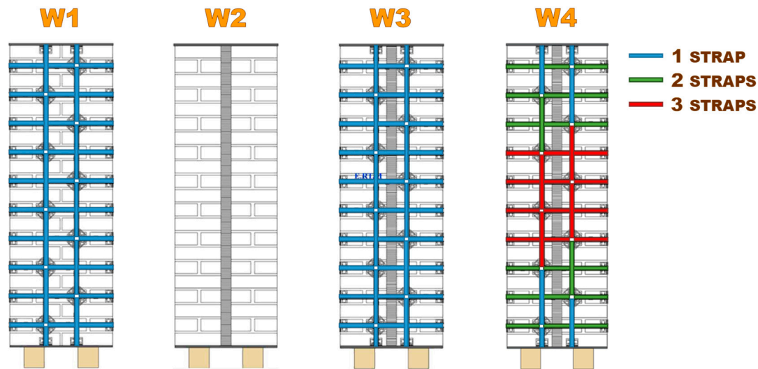
Figure 9. Arrangement of the straps for Specimens W1, W2, W3, and W4.
