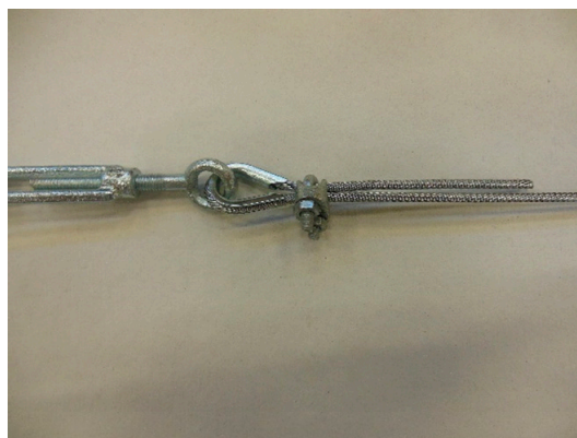
Figure 28. Specimen 3: Flemish eye closed by 1 clip.
