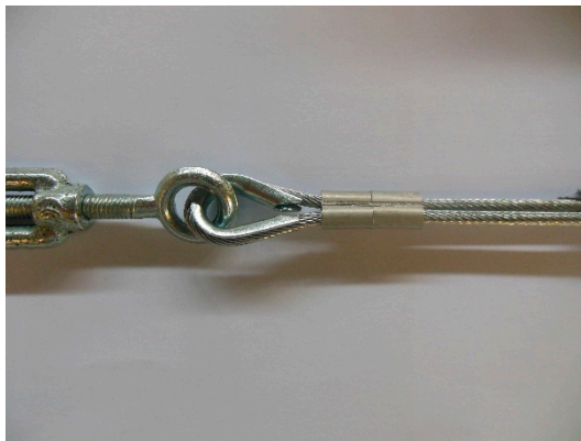
Figure 27. Specimen 2: Flemish eye closed by 2 ferrules.
