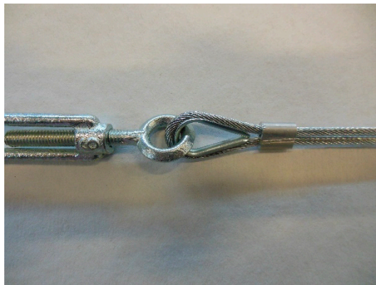
Figure 26. Specimen 1: Flemish eye closed by 1 ferrule.
