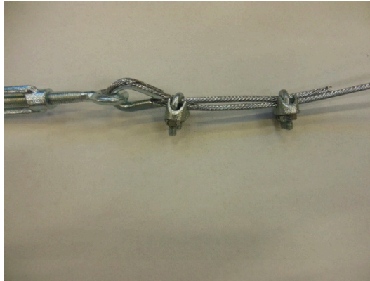
Figure 29. Specimen 4: Flemish eye closed by 2 clips.
