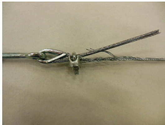
Figure 34. Failure mechanism of Specimen 3.
