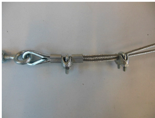
Figure 31. Specimen 6: Flemish eye closed by 1 ferrule, 1 clip, 1 ferrule, and 1 clip, in succession.
