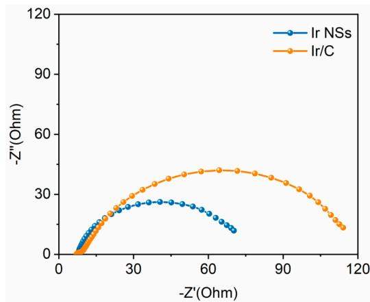
**Figure S3.** EIS of Ir NSs and Ir/C recorded at a potential of 1.53 V (vs RHE).
