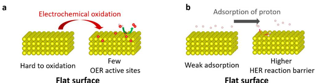
**Figure S9.** Proposed mechanism of OER (a) and HER (b) in flat surface of Ir/C.
