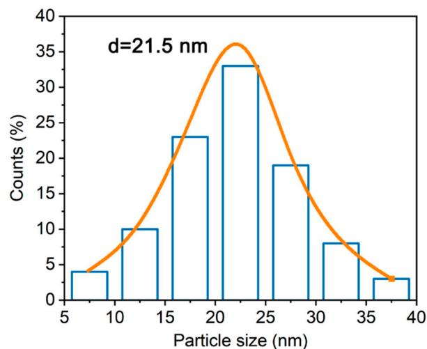
**Figure S2.** Size distribution of Ir NSs. The average size is 21.5 nm.
