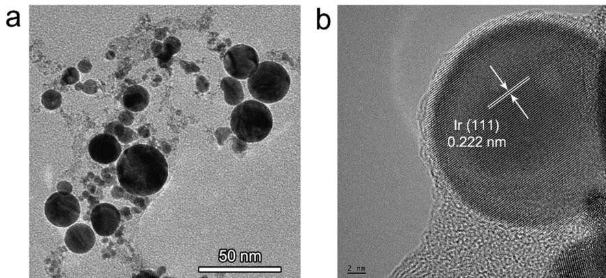
**Figure S5.** TEM (a) and HRTEM (b) images of Ir NSs after HER test.
