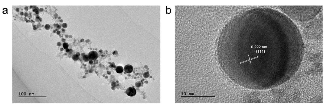
**Figure S4.** TEM (a) and HRTEM (b) images of the Ir NSs after OER test.
