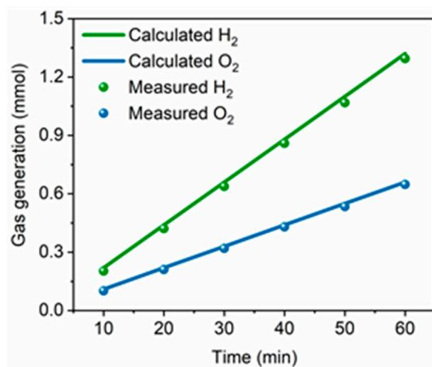
**Figure S10.** Faraday efficiency of the corresponding gas products (O<sub>2</sub> and H<sub>2</sub>) at the current density of 100 mA/cm<sup>2</sup>.
