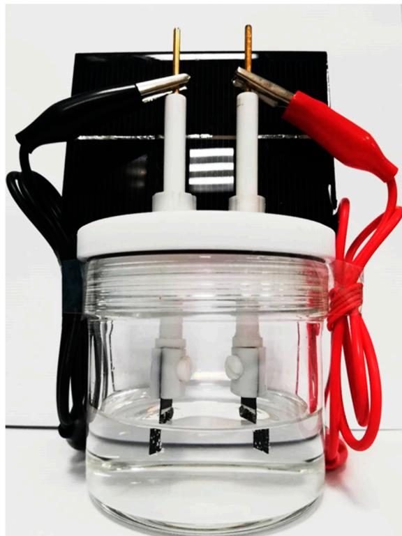
**Figure S11.** Photograph of overall water splitting driven by a 1.5 V solar cell.
