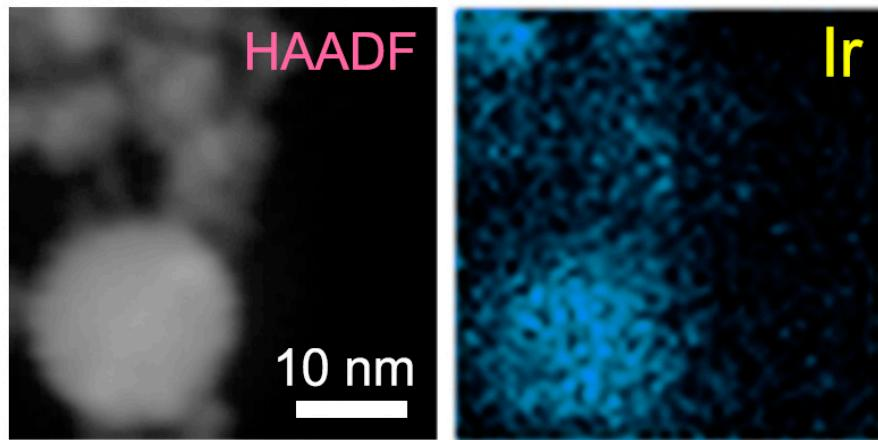
**Figure S1.** HAADF-STEM image and the corresponding EDS mapping of Ir NSs showing elemental distribution of Ir (blue).
