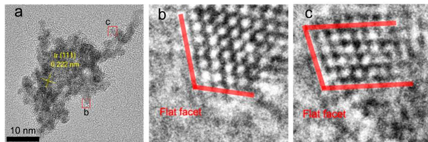
**Figure S8.** TEM (a) and HRTEM (b, c) images of commercial Ir/C.
