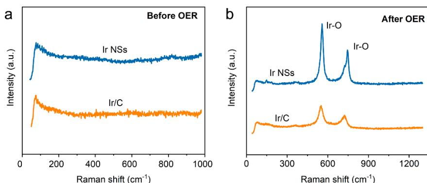
**Figure S6.** Raman shift spectra of Ir NSs and Ir/C before (a) and after (b) OER test.
