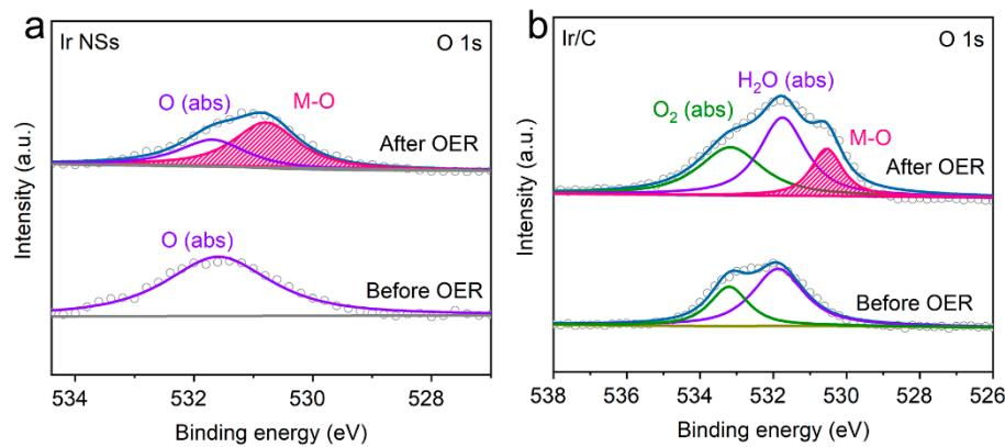
**Figure S7.** XPS O 1s spectra of Ir NSs (a) and commercial Ir/C (b) before and after OER test.
