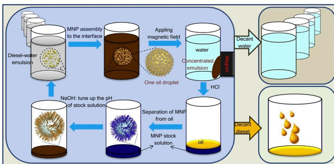
**Scheme 17.** Application of pH-responsive magnetic nanoparticles (MNPs) as recyclable stabilizers for oil–water separation. Reproduced with permission from reference [98].
