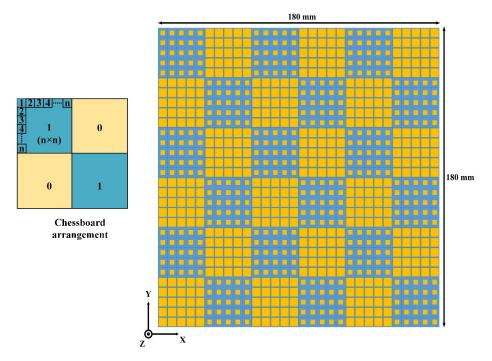
Figure 3. Design of the chessboard-like metasurface.
