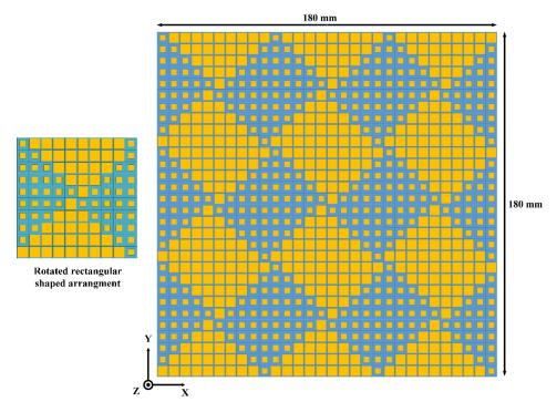
Figure 5. Design of the rotated rectangular-shaped metasurface.
