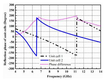
Figure 2. Reflection phase performance of the AMC unit cells.
