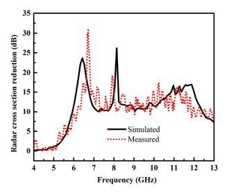
Figure 12. RCS reduction comparison between simulated and measured results.
