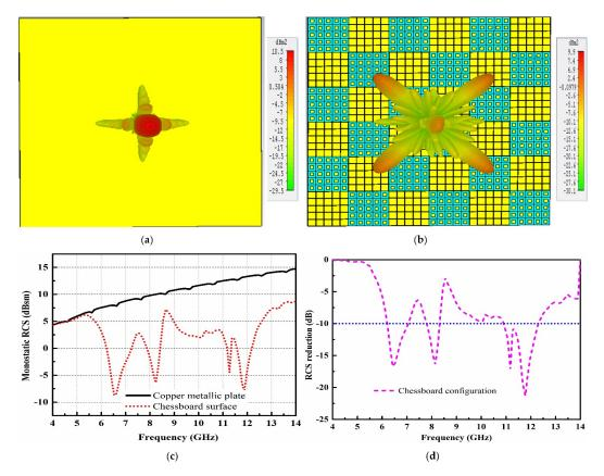
**Figure 4.** Scattering performance of the copper metallic plate and chessboard-like surface. (a) Scattering lobes from the copper metallic plate; (b) Scattering lobes from the chessboard-like surface; (c) Monostatic radar cross section (RCS) performance; (d) The RCS reduction performance.
