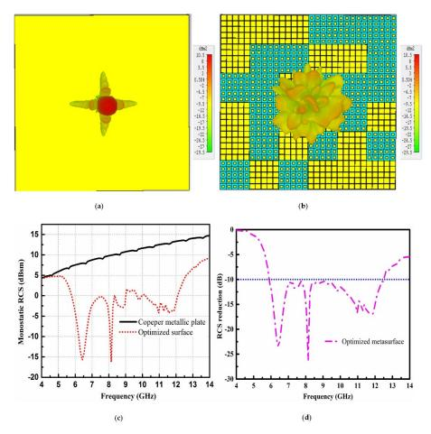
**Figure 9.** Scattering performance of the copper metallic plate and optimized surface. (a) Scattering lobes from the copper metallic plate; (b) Scattering lobes from the optimized surface; (c) Monostatic RCS performance; (d) RCS reduction performance.
