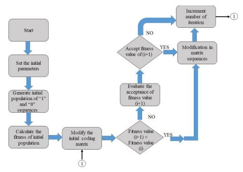
Figure 7. The optimized algorithm.
