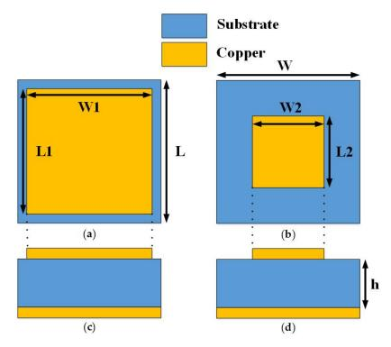
**Figure 1.** The artificial magnetic conductor (AMC) unit cells. (**a**) Top view of the unit cell 1; (**b**) Top view of unit cell 2; (**c**) Side view of the unit cell 1; (**d**) Side view of the unit cell 2.
