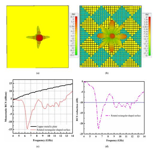
**Figure 6.** Scattering performance of the copper metallic plate and rotated rectangular-shaped surface. (a) Scattering lobes from the copper metallic plate; (b) Scattering lobes from the rotated rectangular-shaped surface; (c) Monostatic RCS performance; (d) RCS reduction performance.
