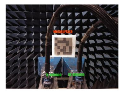
Figure 11. Measurement setup for the reflectivity of an optimized metasurface.
