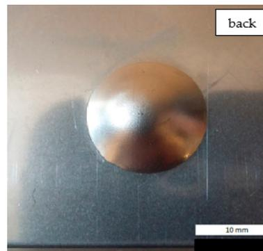
**Table 9.** Coating damage after the impact resistance test.
