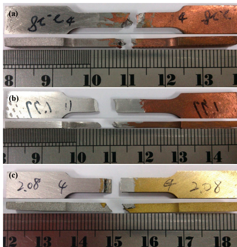
Figure 6. Macrographs of fractured FSW (a) A1/C1, (b) A6/C1, and (c) A1/C2 dissimilar joints after tensile tests.
