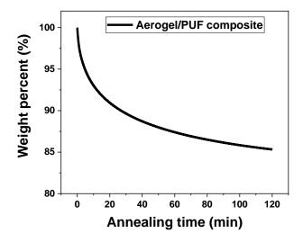
**Figure S1.** Thermogravimetric curve of the GO/CS aerogel/PUF composite thermal treated under 200 °C for 2 h.
