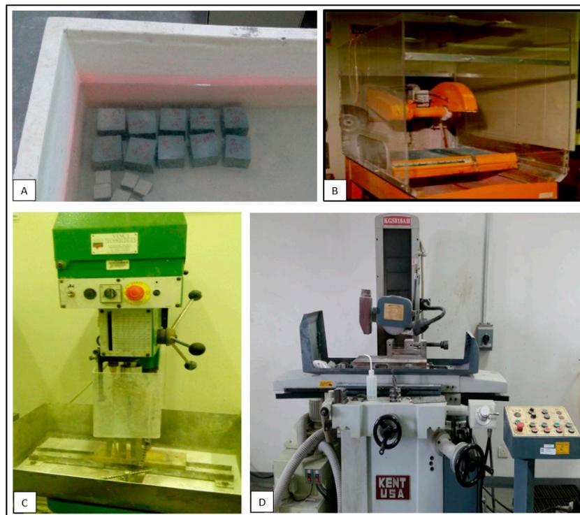
**Figure 1.** Sample preparation phases of cement mortar (A) Curing, (B) Cutting, (C) Coring, (D) End face grinding.
