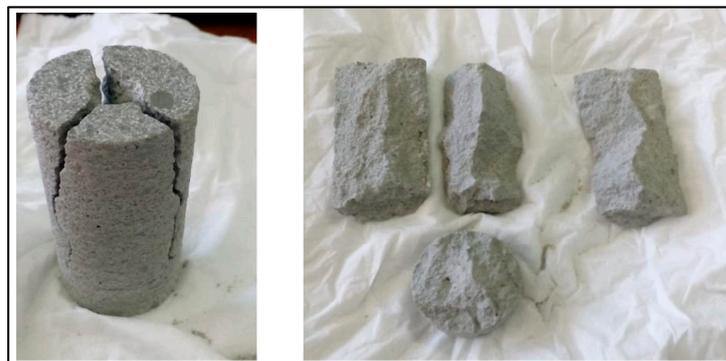
**Figure 10.** Fractured mortar sample after dynamic compression impact loading test (Dry Case).
