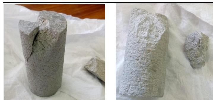
**Figure 11.** Fractured mortar sample after dynamic compression impact loading test (Brine-saturated case).
