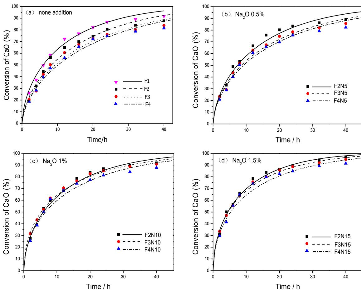
Figure 1. Experimental and simulated absorption rates of CaO under different conditions: (a) None addition; (b) the dosage of Na<sub>2</sub>O is 0.5%; (c) the dosage of Na<sub>2</sub>O is 1.0%; (d) the dosage of Na<sub>2</sub>O is 1.5%.
